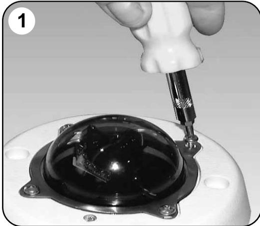
If focus of the camera is needed, access to the series 1000 fixed dome camera is made possible by removing the hemisphere fixing ring, by first unscrewing the 4 x M4 Torx Head screws.
